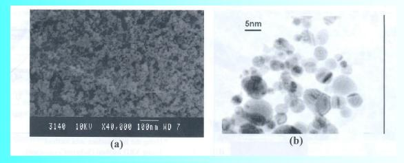
(a) SEM image of MgO nanoparticles (b) TEM image of MgO nanoparticles.
