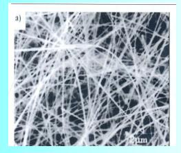
**SEM image of MgO nanowires obtained from the PMT process at 500° C**
