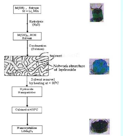
Flow chart for the preparation of LiMn<sub>2</sub>O<sub>4</sub> nanopowder by sol-gel method
